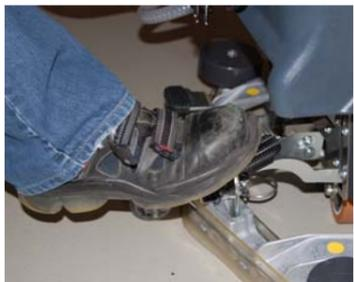
7. Lower brush unit with the foot pedal. Briefly pull the operating lever for brush drive to allow coupling of tool
