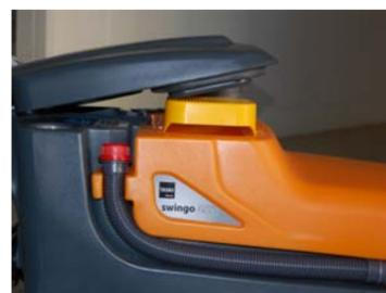
19. Flip the yellow dirt sieve and store the machine with partially open lid for ventilation (lid rests on the yellow dirt sieve)
