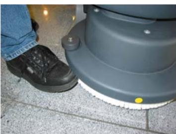
16. Lift brush unit and remove tool by turning anti-clockwise, clean tools and allow to air dry
