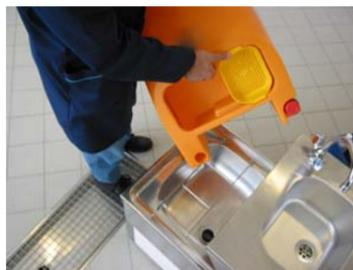
13. Rinse the recovery tank with fresh water. To do so it can be removed from the machine
