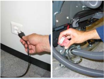
1. Unplug cable of battery charger, then plug red battery cut-off plug into the machine
