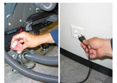
20. Unplug the red battery cut-off plug, then plug in the cable of the battery charger
