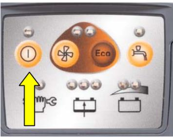
6. Switch on machine with the button on the display – press button for 3 seconds
