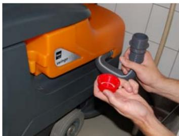
12. Drain recovery tank with the draining hose, then drain the solution tank with the hose on the back-side of the machine
