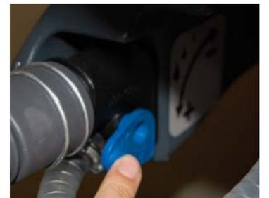
10. Adjust solution flow with the light blue lever on the left side of the machine
