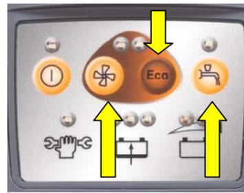
9. Start vacuum motor and solution supply (press orange buttons)
