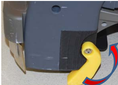
6. Release parking position by lifting machine a bit (parking position is flipping back automatically)
