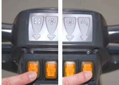
8. Turn machine on (left button), and start solution supply (right button)
