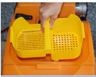
16. Remove water sieves and rinse with water
