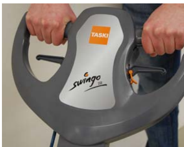
12. Start brush rotation by pressing the levers and clean the floor
