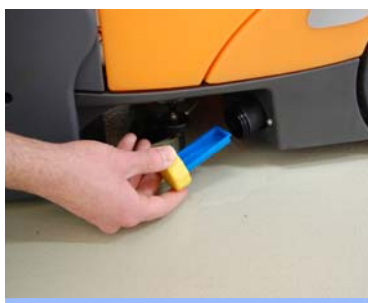
19. Empty fresh water tank and clean solution filter
