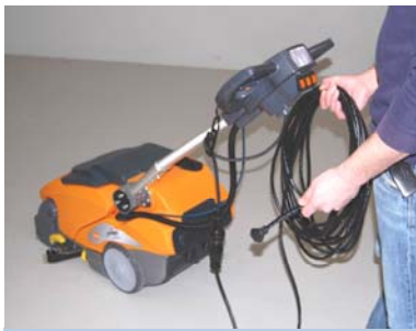
1. Ensure the machine is unplugged and check the mains for damage. If cable is damaged, do not use machine!
