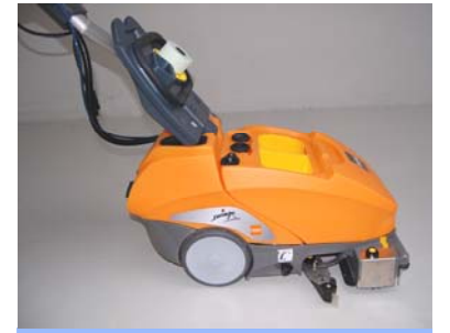
25. Store machine with open lid for ventilation and in parking position.
