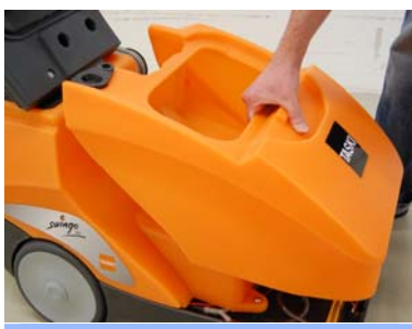
17. Drain, rinse and clean the recovery tank
