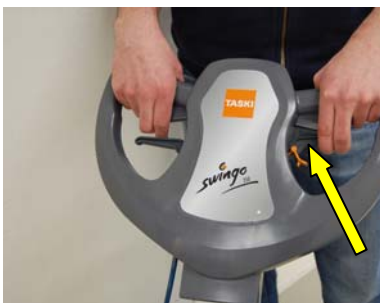
11. Adjust height of the handle (use orange fixation for floated cleaning)
