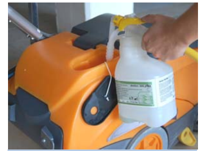
5. or use Diversey cleaning solution dosing system
