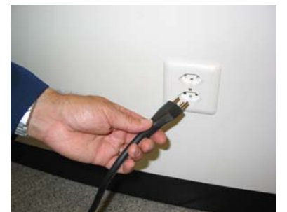
15. Switch OFF all functions of the machine, and then unplug the power cord
