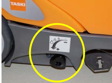
9. Adjust solution flow manually
